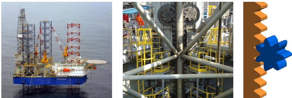
Figure 3.1-1 Left: Jackup platform. Middle: Rack and pinion system on leg. Right: KISSsoft rack and pinion.
