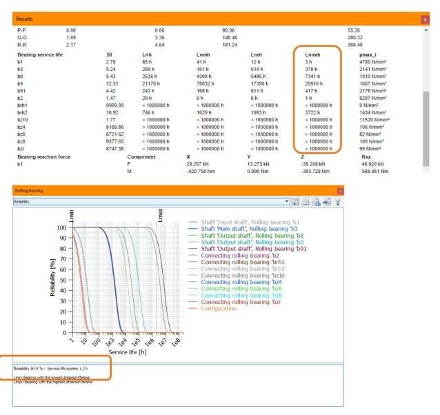
We can see from the results table that bearing b1 has only 3h life and bearing b2 has only 1h life. These two determine the system life.
