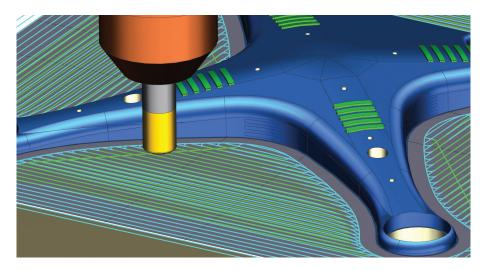
automate machining of many features, including holes, pockets and slots.
