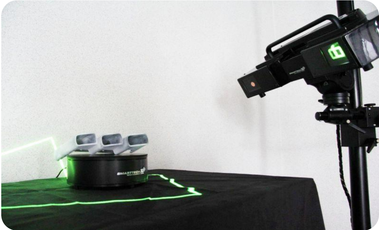
Fig. 3. MICRON3D green 3D scanner while measuring the mountings.
