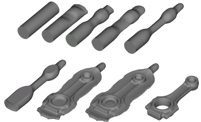
Figure 4: Work-piece shape at end of each operation.
