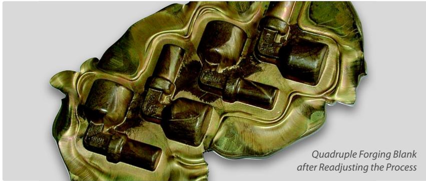
Quadruple Forging Blank after Readjusting the Process
