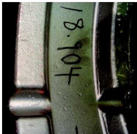
The fold occurred in a critical area and the part had to be rejected
