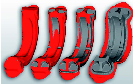
The simulated deformation during finisher using the corrected shape from blocker was formed without lap
