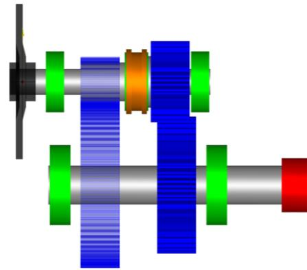
Further development will include the sizing of the synchronizer based on given forces and synchronization time.
