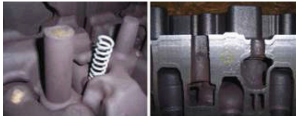
Fig. 6. A metal spring inserted into the core to produce a cylinder head casting serves to provide a high surface chilling device (left). A sectioned cylinder head reveals the remnants of a spring that did not totally melt but fused to the surrounding iron.
