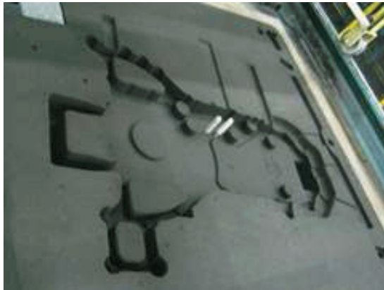
Fig. 7. Two bolts are formed into a large green sand mold as ram-up inserts to force faster solidification into the area.
