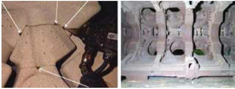
Fig. 5. Holes drilled into cores become chill pins when the mold is filled with iron (left). Clusters of chill pins cast inside the part force those areas to freeze sooner so they are shrinkage-free.
